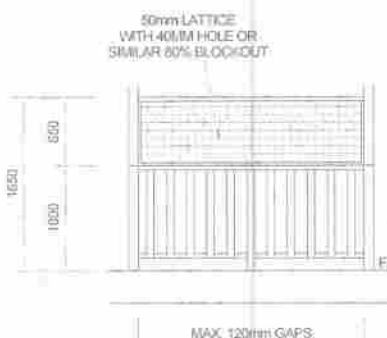
TYPICAL TIMBER SCREEN DETAIL DETAIL 1:50
